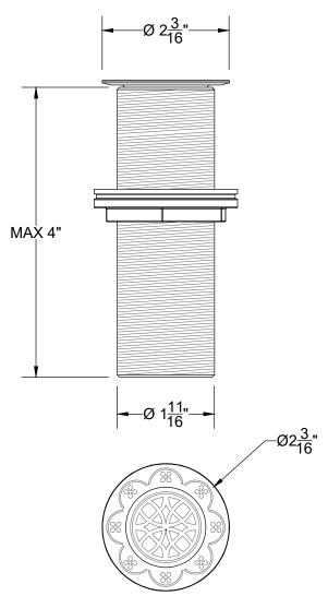
Can be cut for adjustment on site
