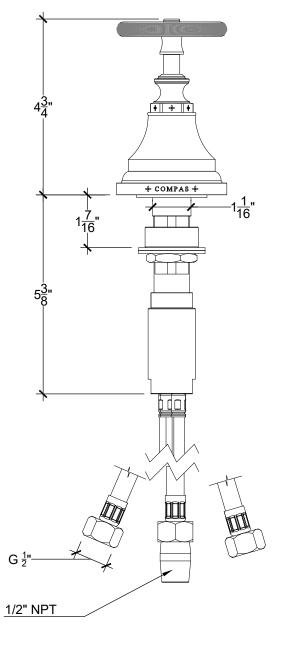
Recommended pressure (3 bar / 45 psi): 13.6 l/min / 3.6 gpm with flow reducer (CA.) 16.2 l/min / 4.2 gpm without flow reducer Prop 65 compliant
