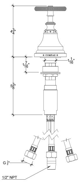
Recommended pressure (3 bar / 45 psi): 13.6 l/min / 3.6 gpm with flow reducer (CA.) 16.2 l/min / 4.2 gpm without flow reducer Prop 65 compliant
