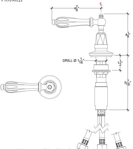
Recommended pressure (3 bar / 45 psi): 13.6 L/min | 3.6 gpm with flow reducer (CA.) 16.2 L/min | 4.2 gpm without flow reducer Prop 65 compliant
