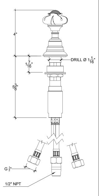
Recommended pressure (3 bar / 45 psi): 13.6 l/min / 3.6 gpm with flow reducer (CA.) 16.2 l/min / 4.2 gpm without flow reducer
