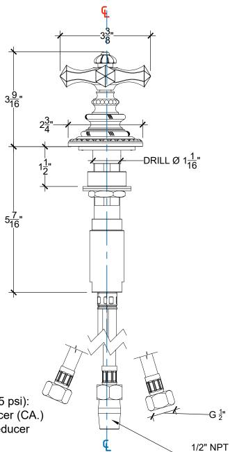
Recommended pressure (3 bar / 45 psi): 13.6 L/min | 3.6 gpm with flow reducer (CA.) 16.2 L/min | 4.2 gpm without flow reducer Prop 65 compliant
